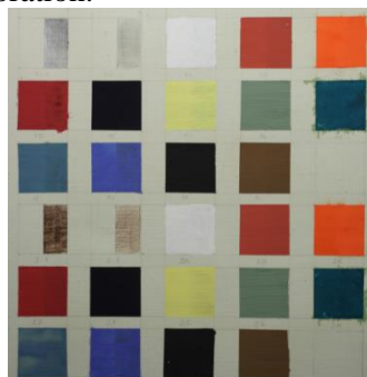
Figure: The canvas with model samples imitating Gothic/Renaissance painting. Transmittance and reflectance of azurite (IR – the canvas, LR, LT - the canvas with azurite layer, JR, JT- the drawing on the canvas).
