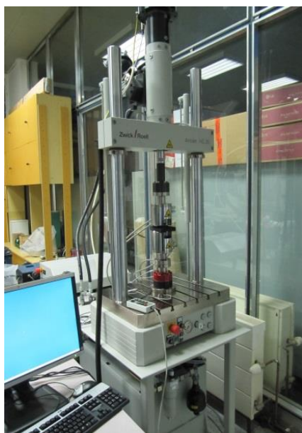
Fig. 4. Servohydraulic testing machine acquired for high cycle fatigue laboratory.
