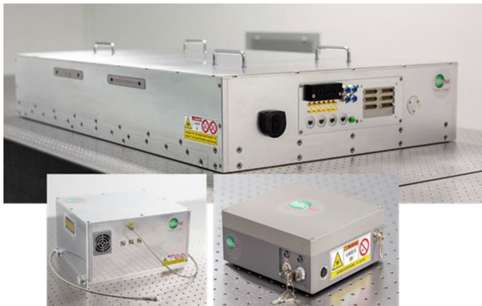
Fig. 8: TRL 6 prototype of the commercial Perla C - 100 laser; 1W fibre-base prototype of a femtosecond front-end (left bottom); GoPico oscillator prototype (right, bottom).
