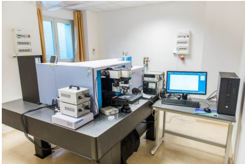
Fig. 2: Raman and photoluminescence microspectrometer LabRAM HR Evolution – HORIBA for characterization of semiconductor heterostructures. (Laboratory of Optical Spectroscopy/LABONIT)
