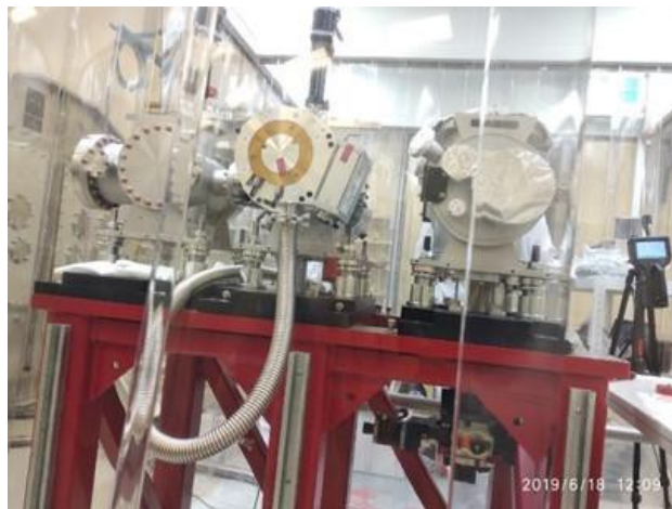
Figure 7: Installation of the LUX components (ELI BL/UHH collaboration) in the E5 experimental hall of ELI Beamlines.
