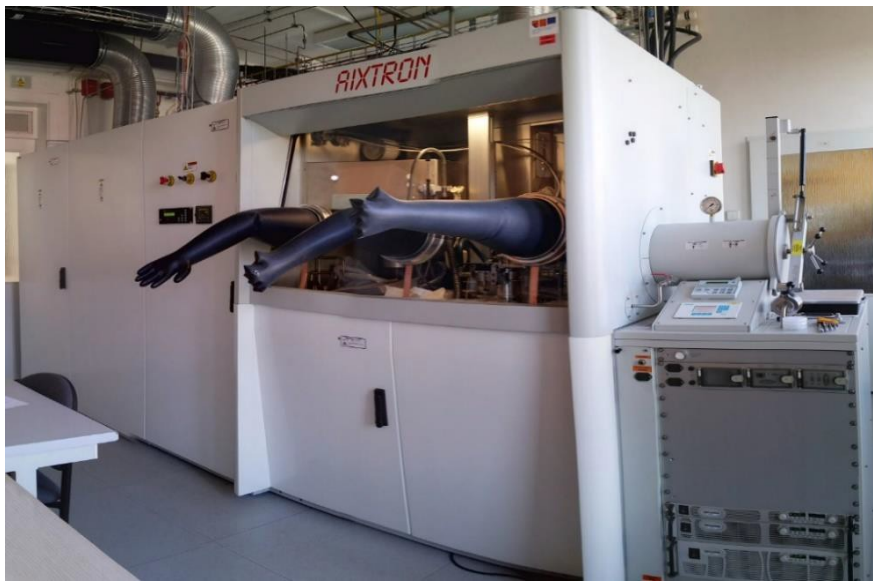
Fig. 1: MOVPE apparatus AIXTRON-CCS 3×2 for the growth of nitride-based semiconductor heterostructures. (Laboratory of MOVPE Technology/ LABONIT)
