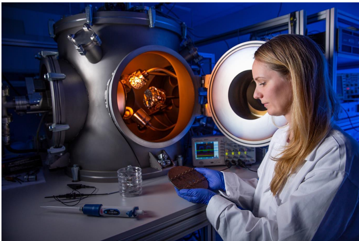
Figure 4: Cold plasma deposition system at the Joint Laboratory of Optics.
