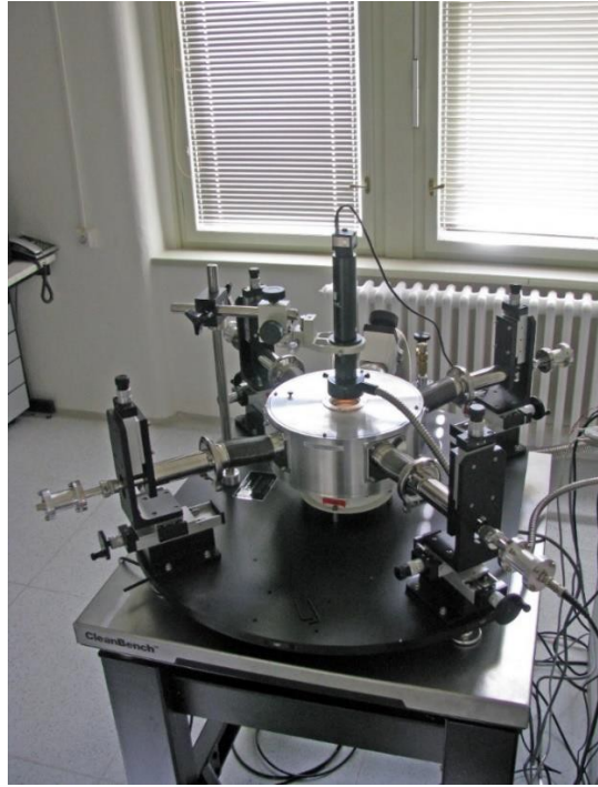
Fig. 5: Probe Station Janis Research ST-500 for transport measurements of small samples in a defined atmosphere and over a wide range of temperatures (5 – 500K). (Laboratory of Transport Phenomena).
