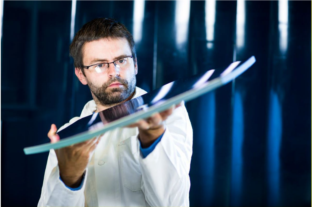
Figure 3: L. Nožka examines one of the mirror segments produced for the fluorescence telescope at the Pierre Auger Observatory.
