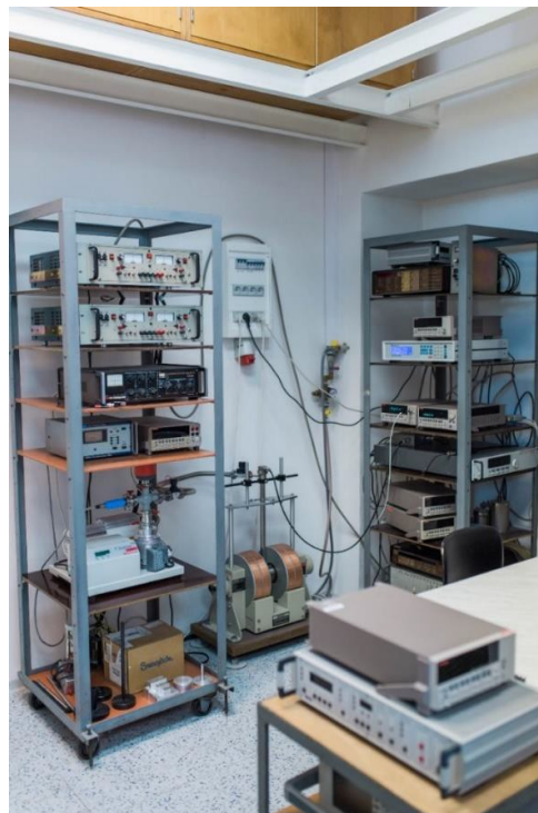
Fig. 3: Equipment for routine magnetotransport characterization of semiconductor structures. (Laboratory of Transport Phenomena)
