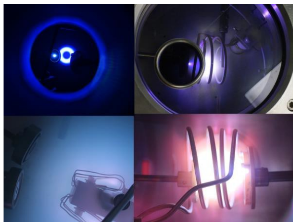
Figure 6. Visualization of the technology processes in the developed PLD-based systems.
