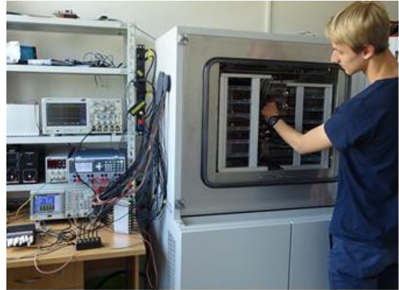
Figure 2 The experimental setup for climate tests of AugerPrime electronics boards in the Prague laboratory in June 2019.
