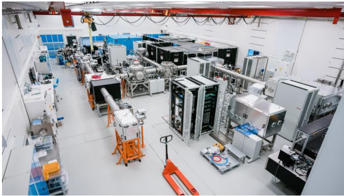
Figure 10: The E1 experimental hall in August 2019. The hall is equipped with a beam transport system that allows the high intensity pulses from the L1 ALLEGRA laser, and the complementary support lasers, to be transported in high vacuum. To the left in the figure are located the HHG source with corresponding VUV science end stations (MAC and ELIps). Centrally, in the blue radiation shielding hutch, are the laser driven Plasma X-ray source and associated experimental stations for X-ray science. On the right is the optical spectroscopy cluster inside the black laser safety enclosure.
