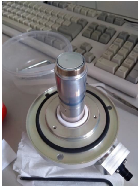
Fig. 9: Light-guide flange of SEM chamber provided at the top with a fast nitride-based scintillator of our design and fabrication.
