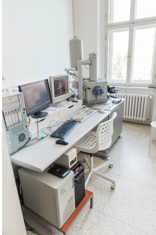
Fig. 4: Refurbished scanning electron microscope Philips XL ESEM TMP with SEM/EDAX/cathodoluminescence facilities. (Laboratory of Luminescence).
