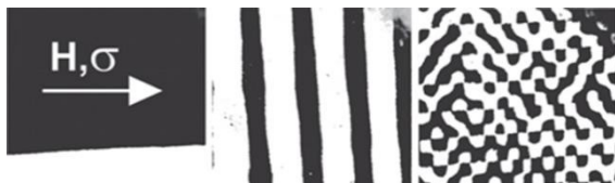
Fig. 6. Magnetic domains in a demagnetized state for compressed Goss-textured (110) [001] Fe-3%Si steel.
