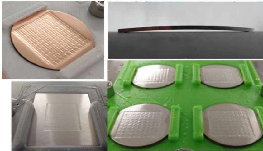
Fig. 12: Examples of materials treated by LSP. Copper for microstructure investigation (top left); aluminium for marine applications (bottom left); cobalt-chrome bending as a result of one-sided compressive stresses (top right); magnesium for bio implants (bottom right).
